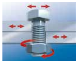
Vibration and loosening.
